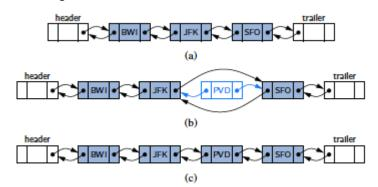
b. If we insert PVD between JFK and SFO, we are either inserting after JFK or before SFO
